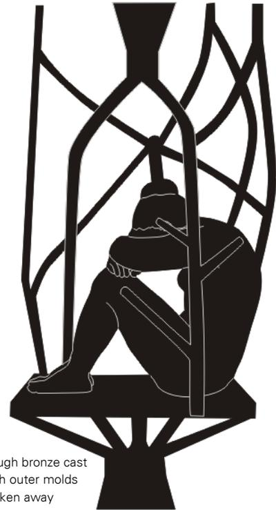
When the bronze is cooled, the outer investment mold is chipped away and the rough bronze is ready for finishing.
